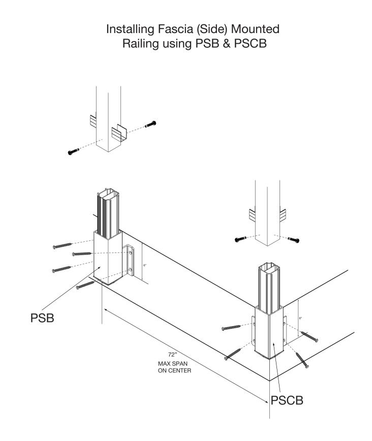
Regal standard deck mounted posts can be adapted to side-mounted posts using our 2 styles of side mount attachment brackets. The PSB can be used to adapt end, line, stair or inside corner applications to side mounted.
